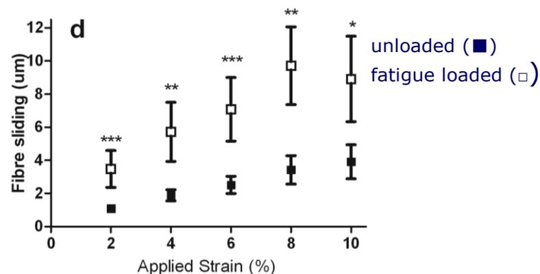
Levels of sliding between collagen fibres increased after repetitive loading in older samples
